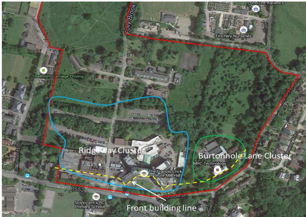
Figure 7 : indicative developable area and front building line
